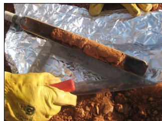
Figure 1.- An example of a soil core (20 x 3,2cm) extracted.
